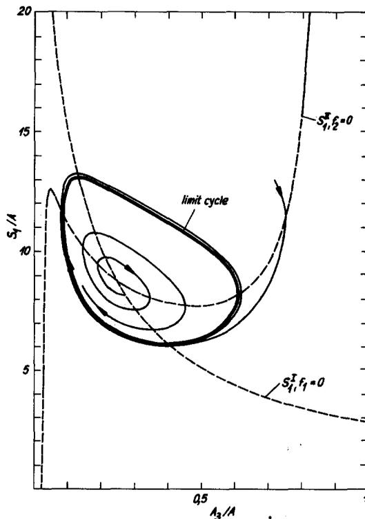
FIG. 36. Trajectories of the stoichiometric model of glycolysis (reaction Scheme 18) which approach a limit cycle. Parameter values:  $v_0/k_1 A^2 = 3.0$ ,  $k_7/k_1 A = 0.1$ . The other parameter values are as indicated in the legend to Fig. 35.
